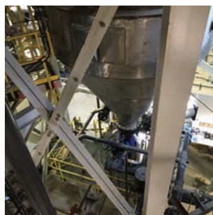
Lower portion of one of the three Ostara Pearl reactors in the phosphorus recovery facility.
